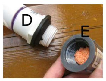
When hand-tightened, the rubber gasket or Teflon tape should keep the connection sealed.
