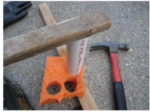
With my plastic punch, I can punch out sponge tips with a half-dozen hammer-blows each. No need to remove each sponge tip — you can wait until you have cut holes in the whole sponge before poking out the whole stack with a stick.
